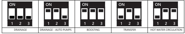
Once dipswitches are set and floats, probes or pressure switches connected, turn internal MCB on, close the cover and connect the power supply. 220, 8
